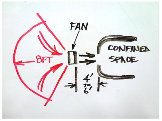
Place duct in horizontal spaces within 10 feet of the far wall.
