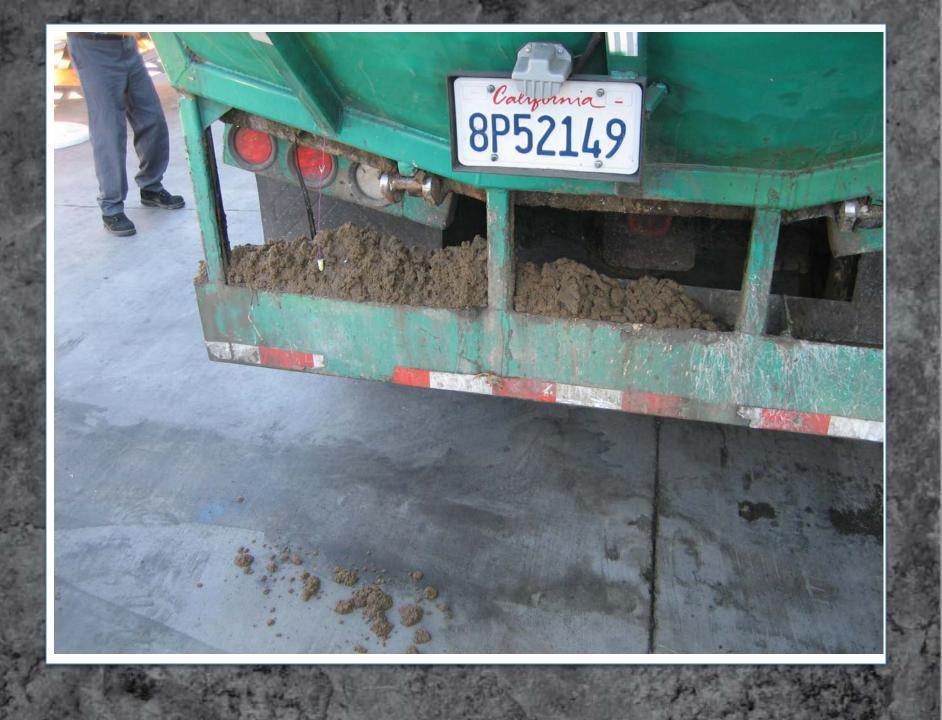
If you decide instead to put your sludge into a roll off dumpster, make sure it can drain to somewhere and place it in a way that when they tilt it to pick it up and several cubic yards of wet, stinky sludge slides into your parking lot you have a way to load it back in besides 2 guys shoveling for 4 hours. And build a big roof over your roll-off so when it rains the EPA doesn't come after you. They hate to see sludge in the storm sewers and creeks.
