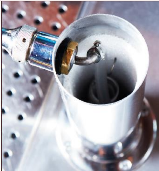
Figure 1.16. Bent tube shank installed in a single-tower kegator.
