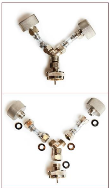
Figure 7.24. Example fittings for constructing a three-way cleaning adapter.
